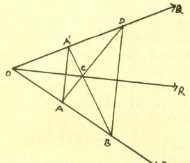
Join AA' and BB'. From Fig.3, We get, OA=OA' - By Construction. OB = OB $\therefore \triangle$  OAA' is an Isosceles Triangle.  $\therefore |OAA'| = |OA'A|$
