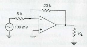
16. For the given differential amplifier circuit, determine the value of output voltage.
