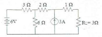
31. Using superposition principle, find the different currents flowing in the branches and voltage across 6  $\Omega$  resistor for the circuit shown below.
