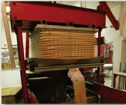
Cold Hollow's rack-and-cloth vertical press
