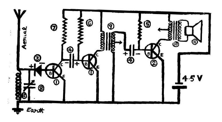
Connections. The connections are done by soldering the components referring to the given diagram. (An electric soldering iron is needed for this)
